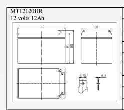
MT12120HR having its design life of 8 years @ 20 degree Celsius for floating application and around 1500 cycles for 30% depth of discharge for cyclic application.
