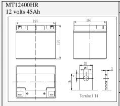
MT12400HR having its design life of 12 years @ 20 degree Celsius for floating application and around 1800 cycles for 30% depth of discharge for cyclic application.
